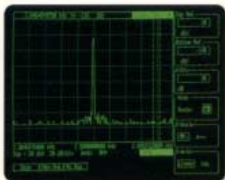
The above trace shows a clean 2.5 kHz signal in a 390 Hz span with no averaging. Any nearby signal, such as 60 or 120 Hz sidebands, would be easily detected at a level of -110 dB below the carrier.
