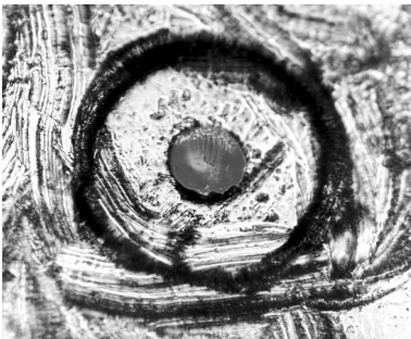
Figure 4-8. Damage from improper cleaning.
